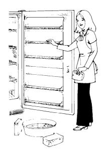
Wash inside of freezer with a solution of 2 tablespoons of baking soda to one quart of warm water. Rinse and dry. Wash the gasket strip around the door with warm, soapy water. Rinse and dry.
